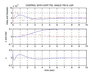
Figure 5. Responses of pendulum angle  $\theta$ , angular velocity  $\theta$ , cart position x, cart velocity  $\dot{x}$ , and control force u of nonlinear inverted pendulum system with Angle PID, Cart PID & LQR Control.
