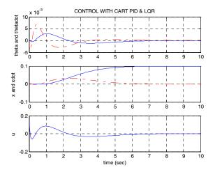
Figure 7. Responses of pendulum angle  $\theta$ , angular velocity  $\dot{\theta}$ , cart position x, cart velocity  $\dot{x}$ , and control force u of nonlinear inverted pendulum system with Cart PID & LQR Control.
