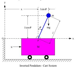
Figure 1. Motor Driven Inverted Pendulum-Cart System.
